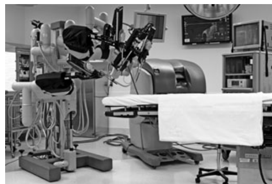
Figure 2 Surgical cart with four robotic arms
