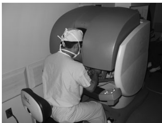
Figure 1 Surgical console of the daVinci system
